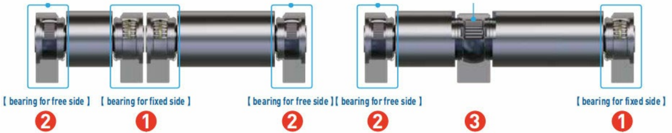
Optimal configuration for roll elongation absorption using single and split rolls
